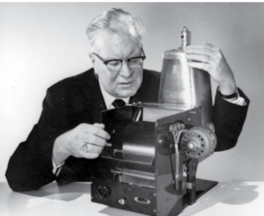
Figure 2. Chester Carlson spent many years (and endured much trial and tribulation) inventing the first xerographic apparatus (left). His patent describing the process, called electrophotography , was issued in 1942 (right). (Images courtesy of Xerox Corporation.)
